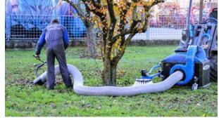
cleaning area. The leaf vacuum is equipped with a floating system and four adjustable wheels that allow to work well on uneven surfaces also. The suction mouth is made of plastic material that can absorbs even small impacts.
